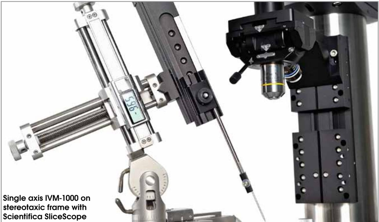
Single axis IVM-1000 on stereotaxic frame with Scientifica SliceScope
