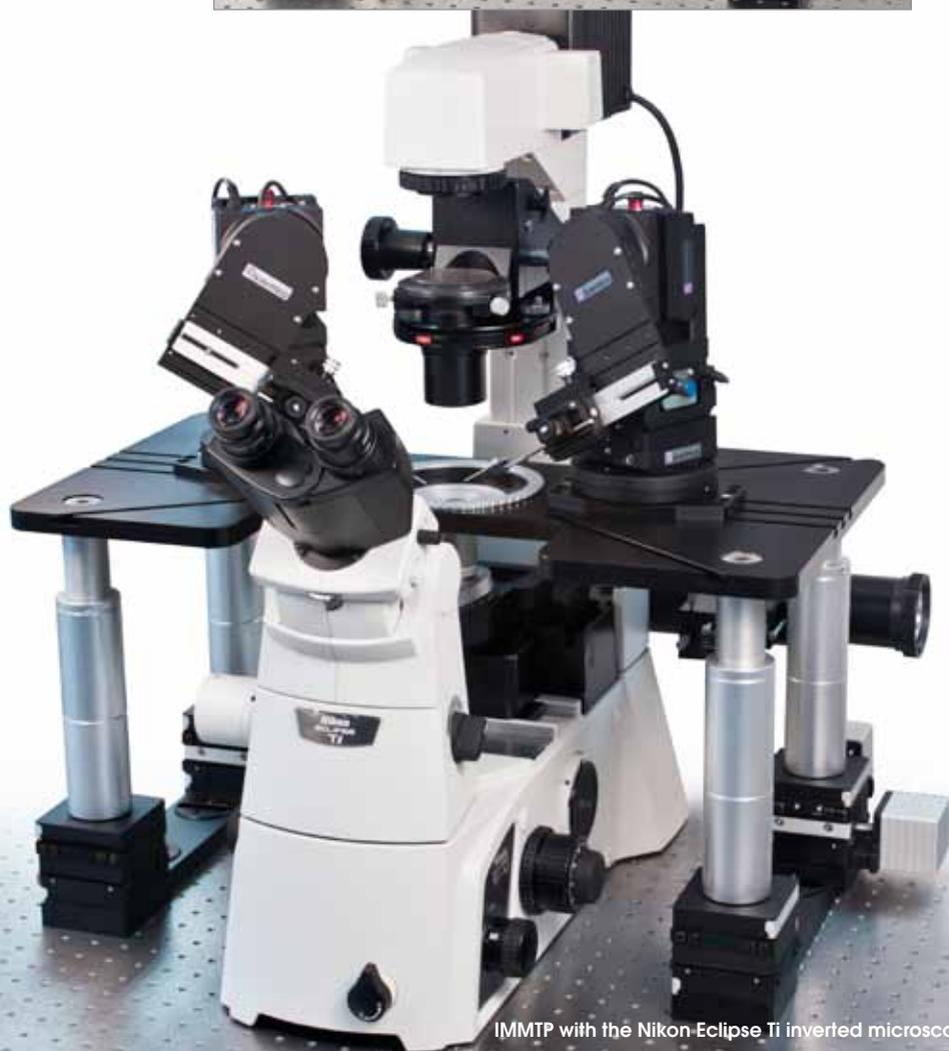
IMMP with the Nikon Eclipse TI inverted microscope
