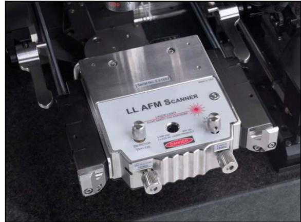
A new, closed loop flexure scanner with ultra-low noise inductive sensors allows for positional precision and accuracy.
